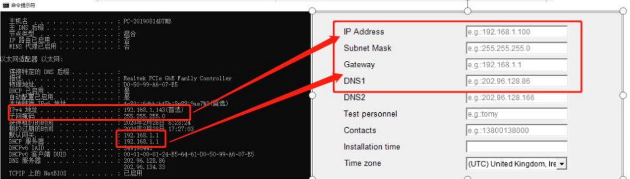
3: After filling out the corresponding data, write the module and complete the IP setting of the 980 network board module :
